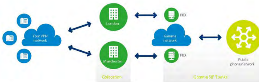
A typical dedicated hybrid hosted PBX implementation
